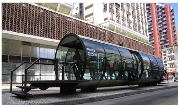
When faced with high ridership problems due to a conventional boarding systems, Lerner created revamped glass tube stations that enabled faster boarding through multiple doors, where passengers pay fares before entering the station. The new "tube stations" opened in October 1991 as part of the first Ligeirinho express line. Today there are 357 tube stations throughout the city.
